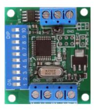
This compact DMX512 to SPI decoder is used to control RGB LEDs driven by either the WS2801 or WS2803 IC in 12V or 5V setups. It can be used with a DMX512 input signal or run as a stand alone controller. In stand alone mode there are 17 programs available.
